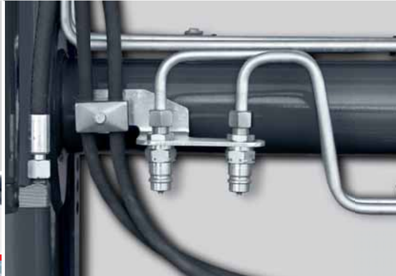
Third control circuit to operate hydraulic tools, e.g. with the gripping function (can be retrofitted on request).
