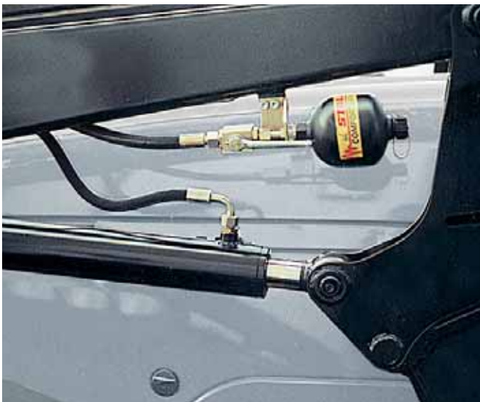
COMFORT-DRIVE: Prevents the tractor from jerking in pitching motions during transport when a front loader is fitted. Protects the driver and the tractor (can also be retrofitted).
