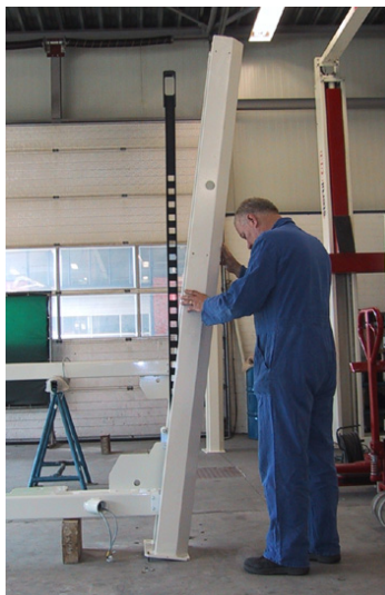
Figure 4.7 Position the locking profiles in the crossbeams
