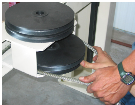
Figure 4.17 Assembly of the steel cables
