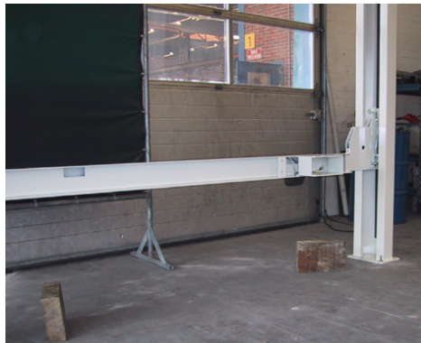
Figure 4.11 Securing the crossbeams at a height of 75 cm
