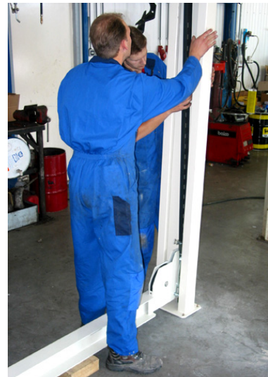
Figure 4.7 Position the locking profiles in the crossbeams
