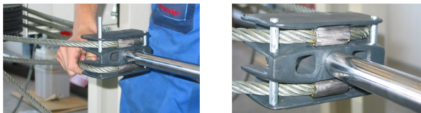
Figure 4.24 Securing the cables to the piston
