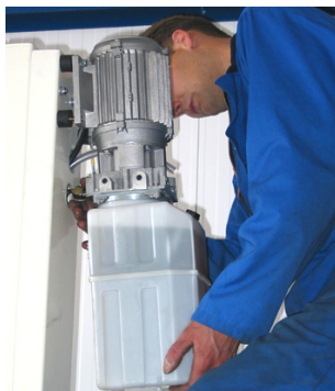
Figure 4.13 Assembly of hydraulic unit
