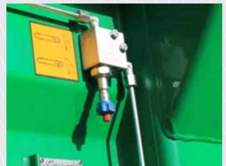
Muck spreaders from SAMSON AGRO can be fitted with a patented hydraulic chain tensioning system (optional extra) that increases the working life of the spreader because it ensures that the chain tensions are always optimal relative to the weight of the material carried in the box. Four cylinders placed in a series ensure a correct tightening of the four chains. The easy use and the controlled tightening of the chains result in low maintenance costs.
