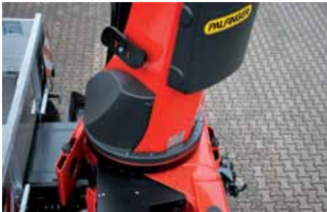
CONTINUOUS SLEWING SYSTEM UNRESTRICTED MOVEMENT
