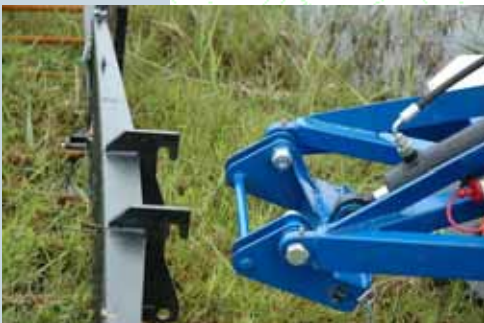
Fast exchange of equipment using a quick-connection attachment .
