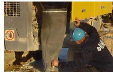
2) Checking dump valve
